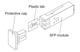
Figure 27. Installing an SFP module into the host port
